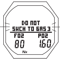
Fig. 103 - GAS SWITCH ALARM
