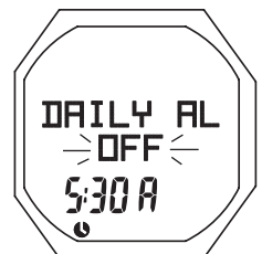
Fig. 15 - DAILY ALARM STATUS (upon access)
