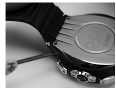
Fig. 166A - TO LOOSEN BATTERY COVER
