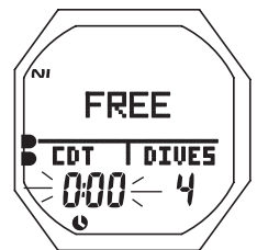
Fig. 129 - SURFACE MAIN (during CDT alarm)
