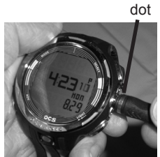
Fig. 162 - PCI CABLE (insert with dot at 12 o'clock)
