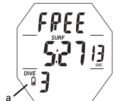
Fig. 2 - LOW BATTERY WARNING
