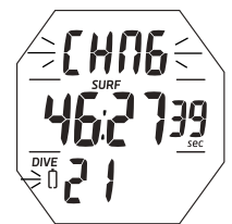
Fig. 73 - FREE SURFACE LOW BATT ALARM
